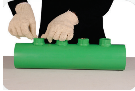
Fuse weld-in saddle with Pipe permanently
